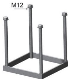
FF 02 HEIGHT: 200 MM Leave 45 MM from top of nut to finished concrete level
