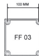
FF 03 HEIGHT: 120 MM Leave 35 MM from top of nut to finished concrete level
